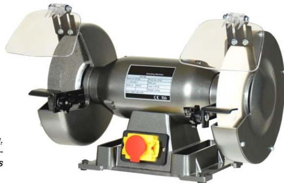
Figure 1-11. Grinding is a cutting operation, like turning, drilling, milling, or sawing. However, instead of the one, two, or multiple-edge cutting tools used in other applications, grinding employs an abrasive tool composed of thousands of cutting edges.
