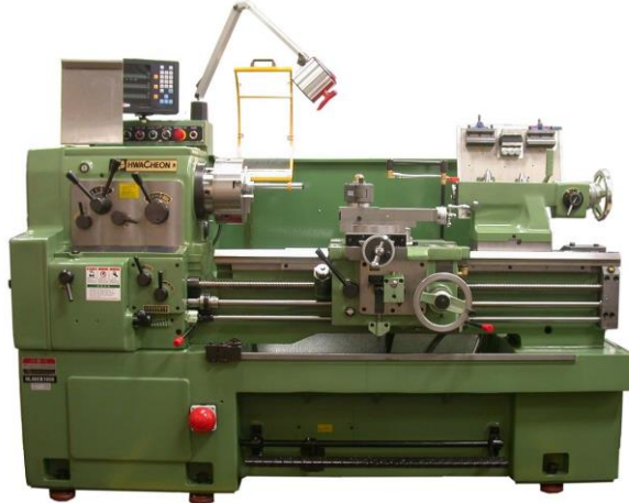
Figure 1-7. The lathe operates on the principle of the work being rotated against the edge of a cutting tool.
