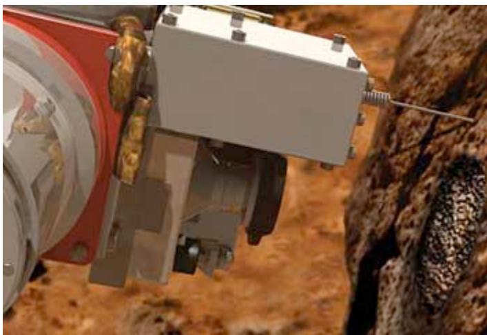
The Rover arm carries four instruments that collect data about the surface of Mars.
